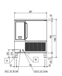
Drain Electrical inlet (power) ΕI Refrigerant Outlet
